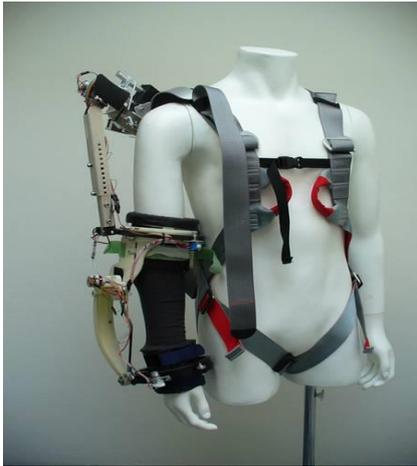
The passive exoskeletons use passive elements such as springs, dampeners etc., to transfer the payload to the ground, however active exoskeletons not only transfer the payload to the ground but also impart energy through the actuators resulting in reduced energy consumption by the soldier,
